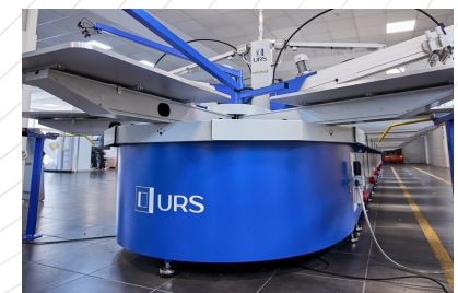
Communication and energy connection sockets near the printheads for flash cure
