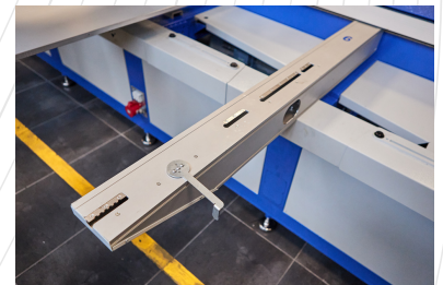
Easy demountable pallet carrier systems
